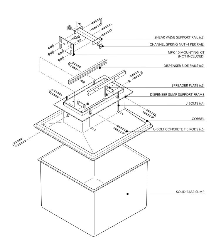
$682 mm \times 682 mm$  GRP solid base sump and corbel to fit 1 hose, 2 hose & 4 hose Gilbarco Electroline Dispenser. Pressure System.
