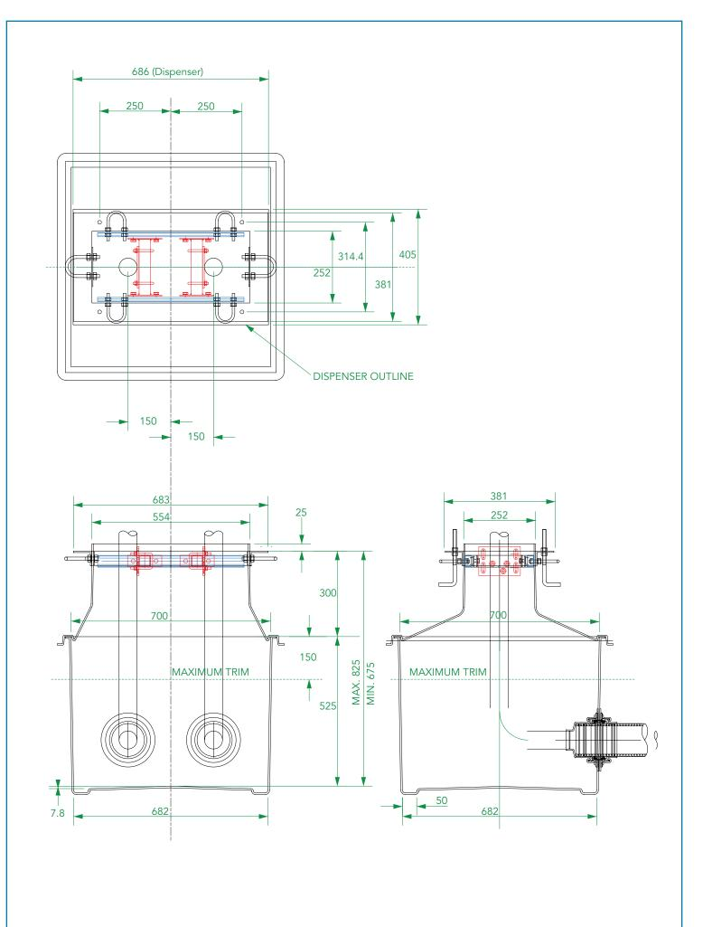
682mm x 682mm GRP solid base sump and corbel to fit 1 hose, 2 hose & 4 hose Gilbarco Electroline Dispenser. Pressure System.
