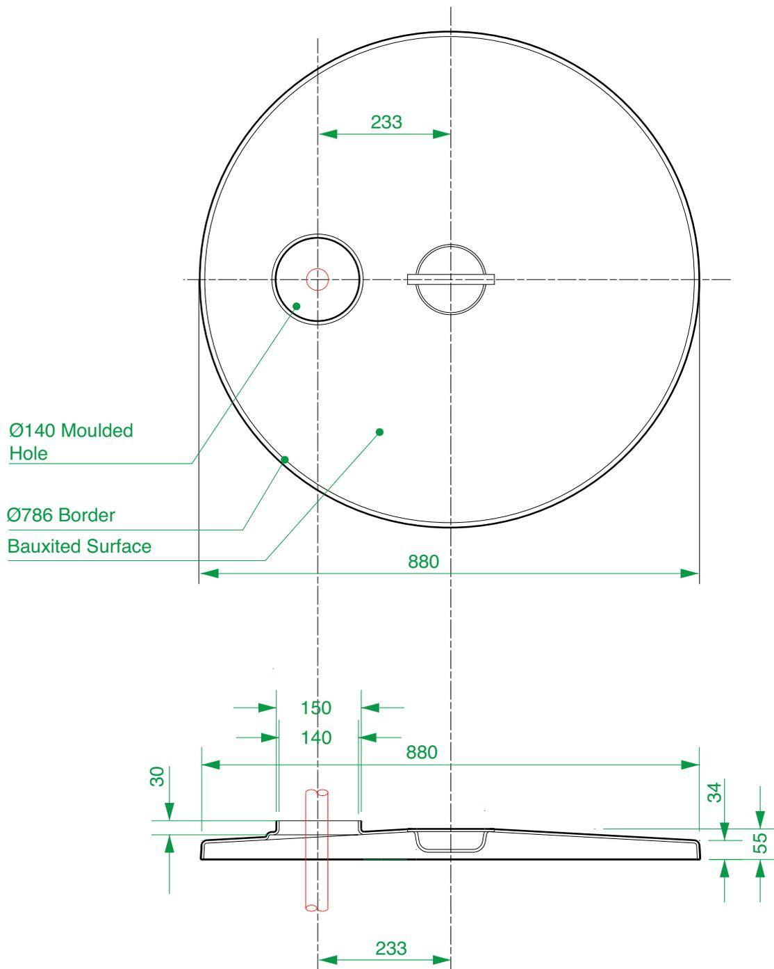
Structural platform with moulded offset sealed port for manual dip stick. Fits all chamber systems with FL90 cover. Anti-slip surface.
